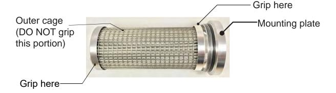
In this situation, grip the primary filter media assembly by the base (do not grip the filter by the outer cage) carefully unscrew the primary filter media assembly from the mounting plate (turning counterclockwise).
