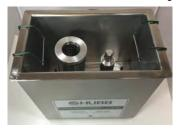
4. Add tap water to fill line in cleaning station or just enough to cover filters. (HOT tap water is preferred).
